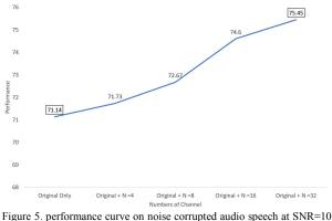
Figure 5. performance curve on noise corrupted audio speech at SNR=10 dB tested with the original data set and the augumented data sets. From let to right, "Original Only" means training with 100% original dataset, "Original + N =4" means trianing with augmented dataset (50% original dataset plus 50% 4-channel vocoded speech), and the same mixing strategy for N=8, N=16, and N=32.
