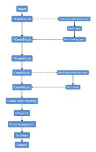
Figure 3. Overall CNN architecture used in this paper. Each \*ConvBlock is followed by a batch normalization layer, a ReLU layer, and a maxpooling layer. Each ConvBlock is followed by a batch normalization layer and a ReLU layer. Global max pooling is followed by the second ConvBlock.
