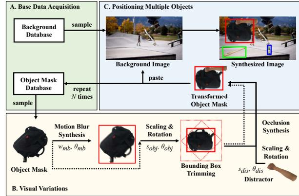
Fig. 2. Overview of the synthetic data generation framework with motion blur and occlusion synthesis. The dotted line transitions occur with 0.5 probability which skips the motion blur or occlusion synthesis stage.
