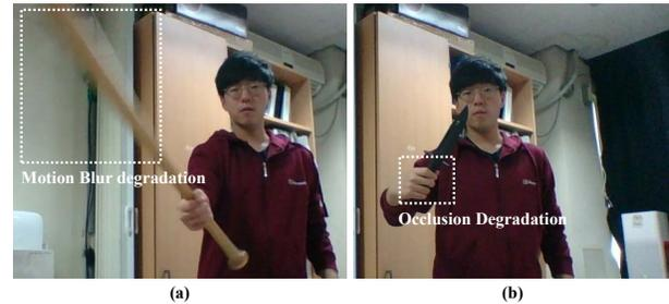
Fig. 1. Two typical types of visual degradation that commonly occur in real-time AR applications. (a) Motion blur (b) Occlusion.
