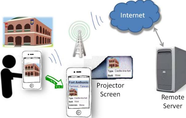
Fig. 4 Overview of the proposed vision-based navigation system.
